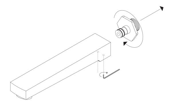
2 - For a succesful installation, the female in-wall connection needs to be flush with the finished wall surface. Use the appropriate length male nipple to make this true. Apply teflon tape to the threads and install.
