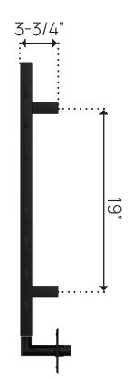
Bottom of frame to center of electrical box
